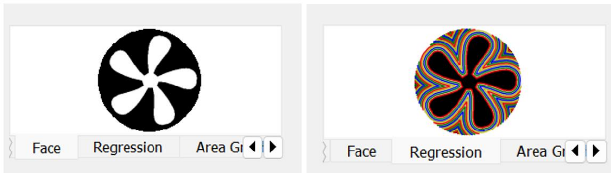
Figure 2: The Face and regression patten of my custom propeller port in the openMotor UI
